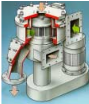
Fig. 8: Centrifugal classifier w/mechanical dispersion
