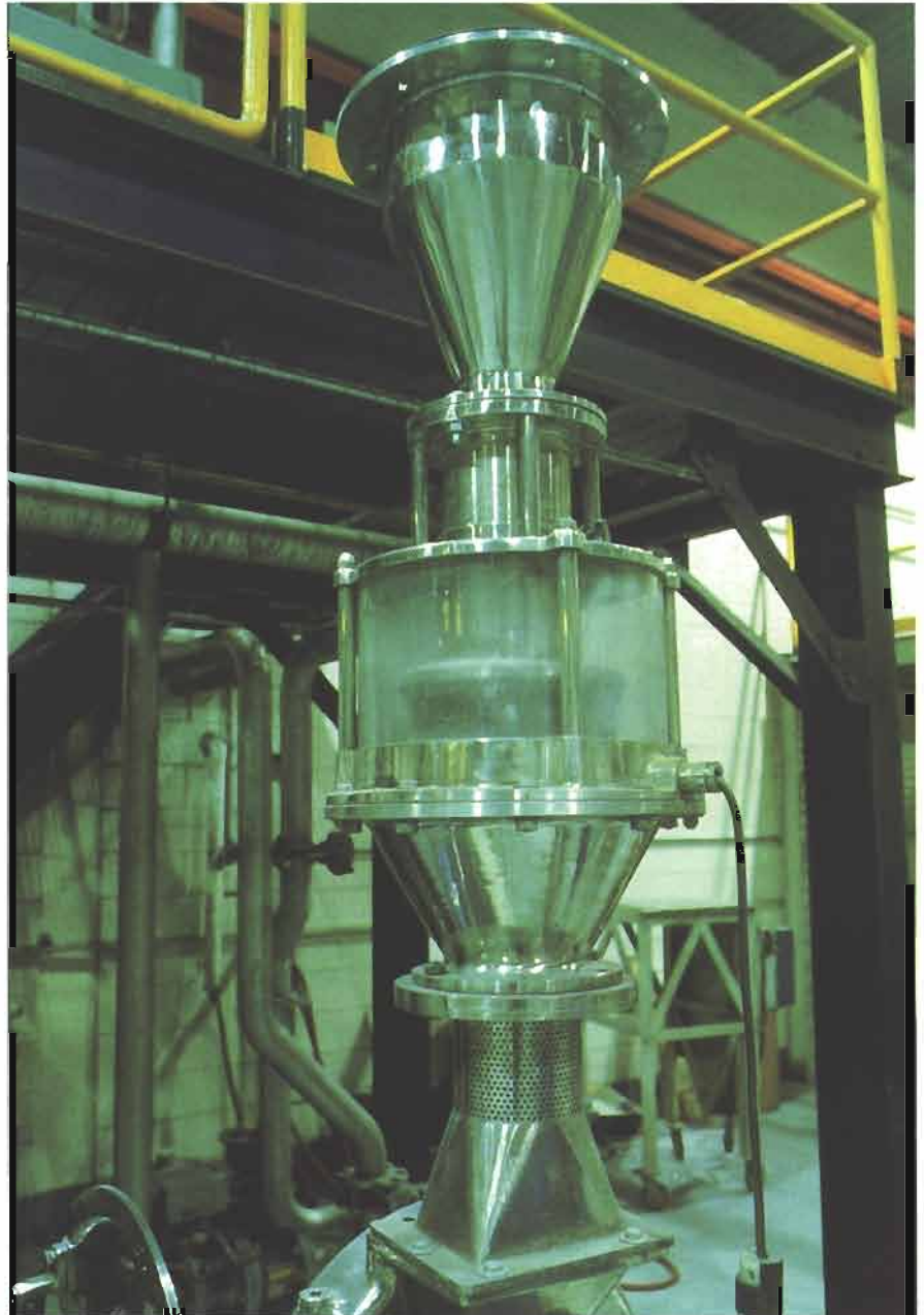
A mechanical impact mill in the test center (mounted beneath a feeder) performed toner milling prior to final grinding and double classification.
