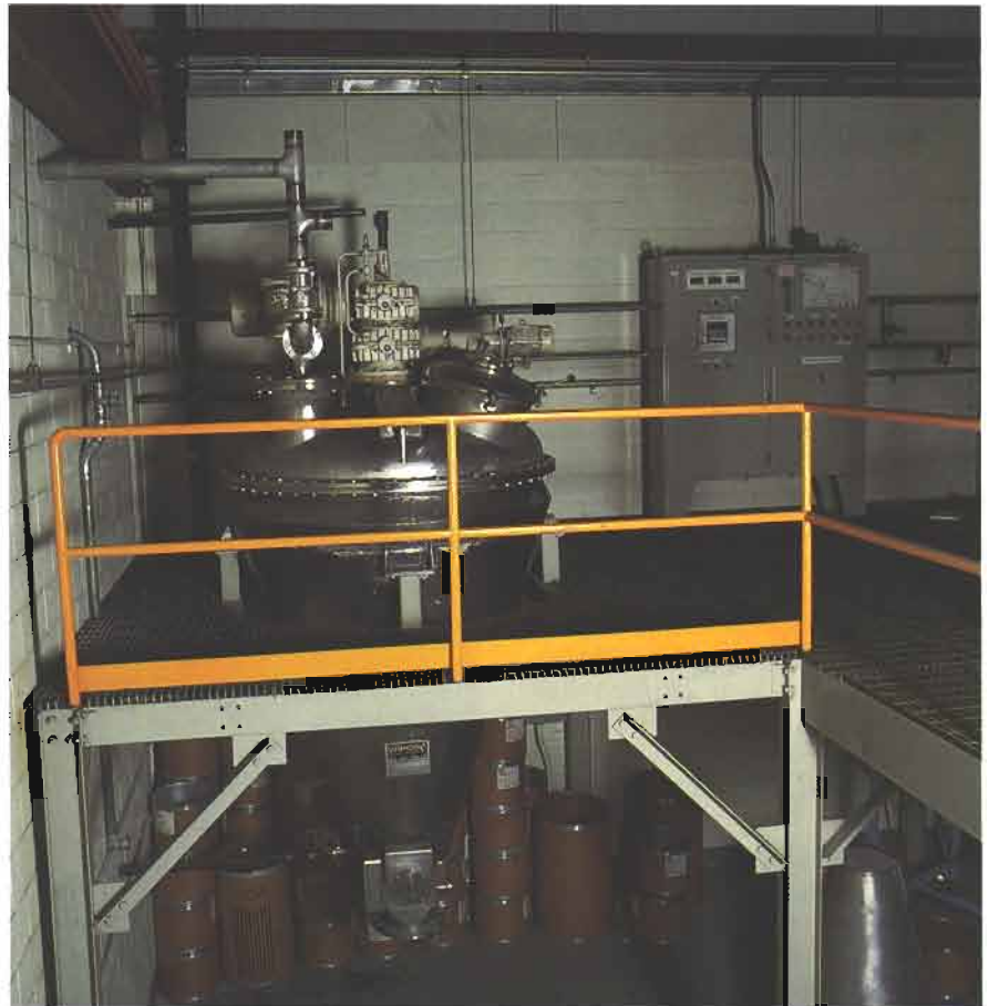
A conical screw mixer in the Micron Powder Systems test center combined toner ingredients without generating excessive heat.
